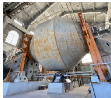
The cable hoist drum of the 1920 Norberg Steam Hoist, at Quincy Mine and housed in a 5-story building, is an enormous spool that held 2.5 miles of 1 5/8 inch diameter steel cable. The spool was a 250 ton, 30-foot-diameter monster - powered by two compound steam engines with cylinders three and five feet in diameter. The cable ran from the Hoist House to the Shaft/Rock House and down the main shaft to the horizontal tunnels. It could raise a 10 ton load at a speed of 36 mph from an inclined depth of 9260 feet (1.5 miles). The hoist was designated a National Historic Mechanical Engineering Landmark in 1984. (K. Clover)
