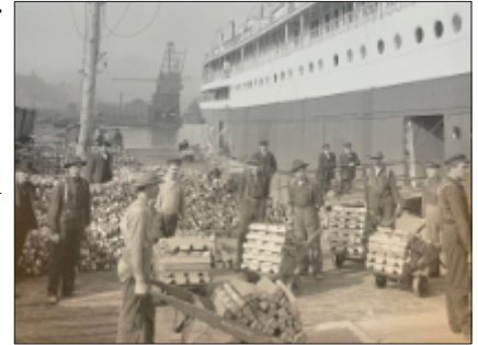
Copper ingots being loaded ~1910 in Houghton, onto Steamboat S.S. Juniata, which was launched in 1904 and initially carried passengers and freight between Buffalo and Duluth. The copper ingots were pure enough to be fabricated into copper products such as wire. (Photo displayed at the Copper Range Depot Restaurant in Houghton, Michigan.)
