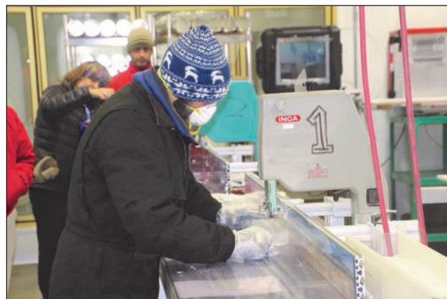
Slicing an ice core for samples
