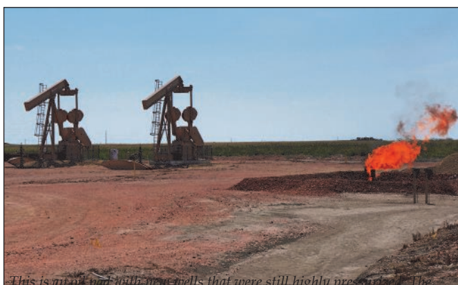
This is an oil pad with new wells that were still highly pressurized. The nodding donkeys are in place, but not operational yet; the natural gas flare burns 24/7.
