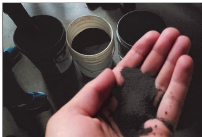
Frack sand in three different particle sizes. We got to touch them to feel the difference and to feel how clean the sand is. Sure enough, there was none of the normal sand dust on my hand after I put the ceramic frack sand back.
